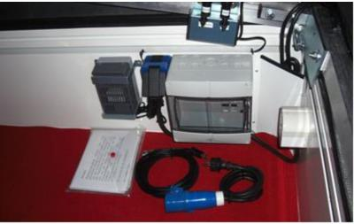
In the storage box at the trailer's front: The junction box (T), inside is the circuit breaker and the safety switch. On its side, the 220volt outlet (S) and the Dryfit charger (Z). See on top the plugs (I) to switch from solar to net charging. Here you can decide if you want to charge from the net or from the Solar system. And if you want to use the charging cable inside or outside of the trailer.
