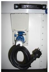
The "IN" plug (U) for 220 (or 110) volts at the trailer's front. With cable (V) and plug. Applies VDE.
