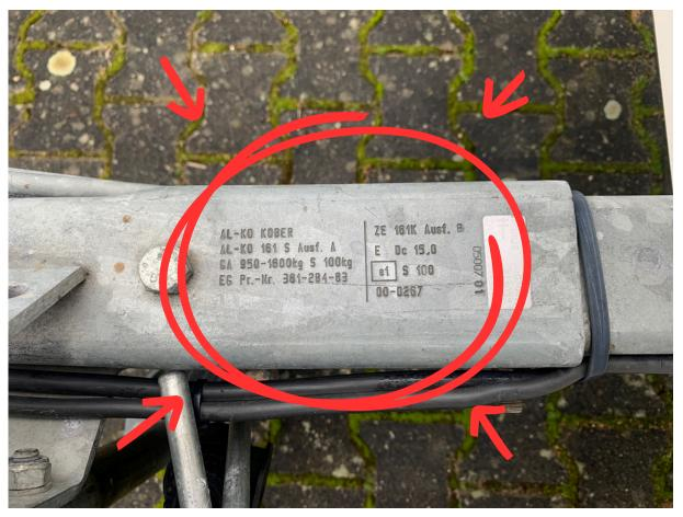
In the case of a round drawbar, the important information is located underneath on the "tag"
