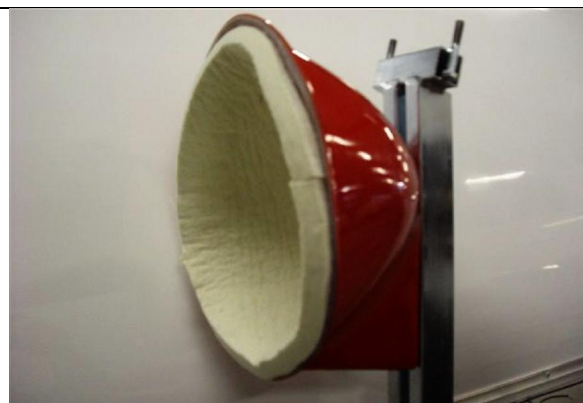
The nose holder for the fuselage: GRP . moulding padded with 20 mm of white sheep felt (standard)
