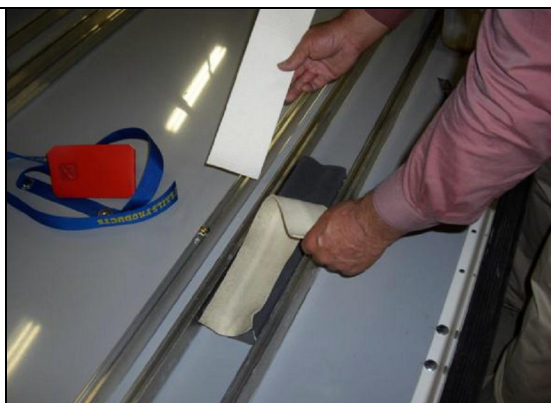
The wing nose rest: easy to change top layers of natural white felt always protect the surface of your wings (standard, spare felts part no 354)
