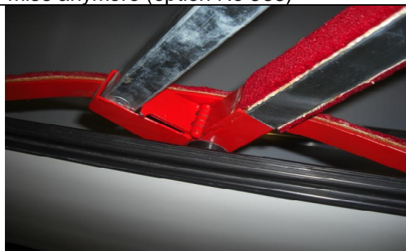
With a click of your finger you activate the second pair of lift arms by switching a hinge.
