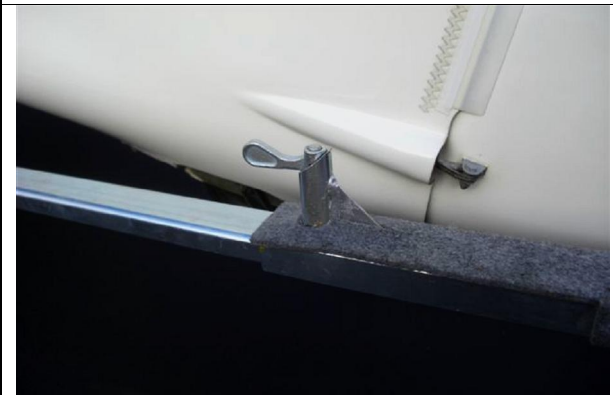
...and the spring loaded lever will lock the telescope automatically.
