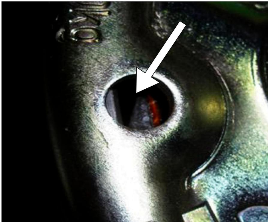
Through the outside hole you can inspect the condition of the brake lining. If the lining is worn to the end of the chamfer, it has to be changed because it is **not possible any more** to adjust the brakes.
