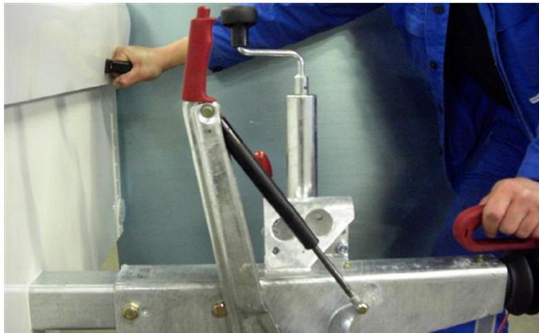
**Test:** Activate the hand brake and push the trailer back by hand .
