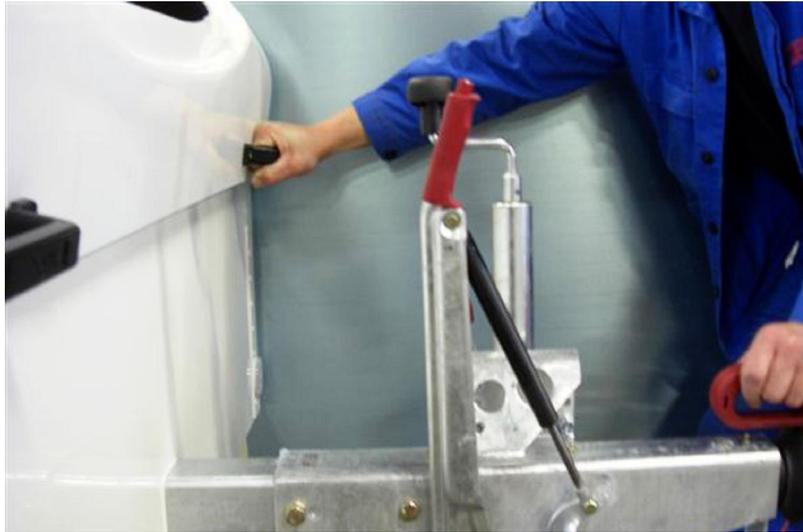
After the trailer is on its wheels again, please check the correct adjustment. Activate the hand brake and push the trailer back by hand. During you are pushing the lever has to move back from itself until it is **90°** to the tongue ( **not more than 90°** !)
