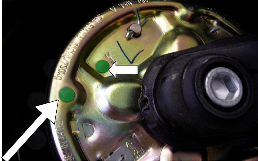
Open both the green plugs on the brake plate with a small screwdriver (rear of the brake drum).
