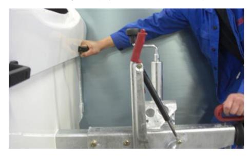
After the trailer is on its wheels again, please check the correct adjustment. Activate the hand brake and push the trailer back by hand. During you are pushing the lever has to move back from itself until it is 90° to the tongue (not more than 90°!).
