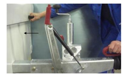
**Test:** Activate the hand brake and push the trailer back by hand. If the hand brake lever – as seen on the picture – moves back more than 90° it is time to adjust the wheel brakes. Lift the trailer and secure with stands! Release the hand brake lever to the front/down (brake open).
