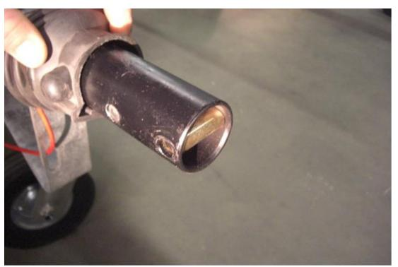
Make sure, that the bushing for the front bolt stays on his place as seen on the picture. The steel pin is still inside the rear hole of the tube to hold the overrunning damper in position.
