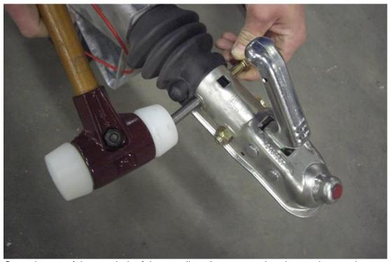
Open the nut of the rear bolt of the coupling. As seen on the picture above, take a steel pin with a diameter of 12 mm, 48 mm long for 161 S or K overrunning brakes, 33 mm long if a 90 S or K overrunning brake is installed. Use this steel pin to push the rear bolt out.
