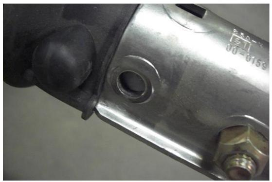
Push this steel pin as far inside the tube, as it allows to take the coupling away while it stays in. This steel pin holds the overrunning damper in his position during the change of the coupling. Disassemble the front bolt.
