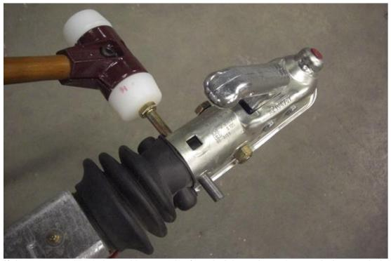
If the new coupling is in position, put the front bolt in and use the rear bolt to push the steel pin out. Make sure that both nuts are to be tightened with a torque of 8,5 kp/m.
