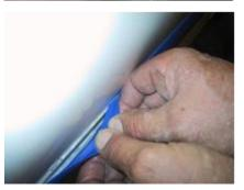
Cut the trim as long it is hot with scissor and knife. Rivet it to the old holes.
