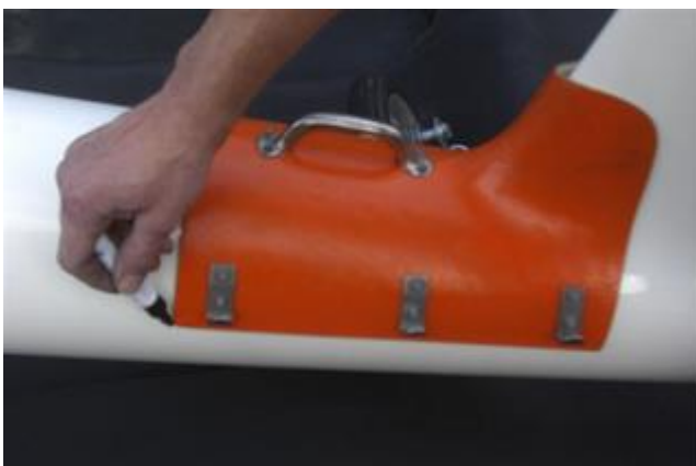
Before the first use mark the front position of the tail dolly at the fuselage. Now you always know exactly where to attach the lifting device.
