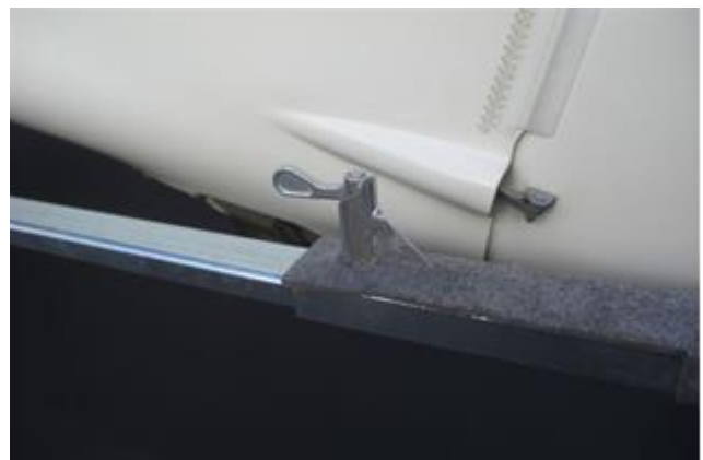
...and the spring-loaded lever will lock the telescope automatically.
