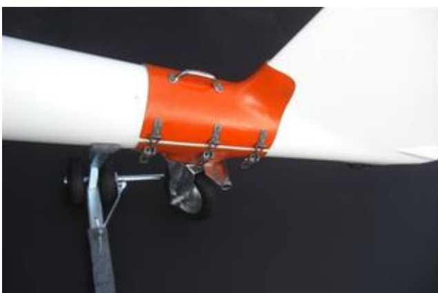
Attach the tail dolly. Lower it to the ground...
