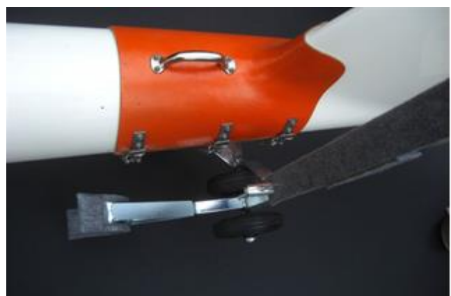
... and plug the pin of the tow bar into the tube at the dolly in a vertical position.
