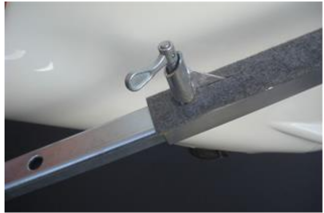
...and check the locking of the bolt head at the tube. Open the spring-loaded lever and move out the bar.
