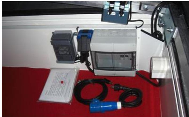
In the storage box at the trailer's front: The junction box (T), inside is the circuit breaker and the safety switch. On its side, the 220-volt outlet (S) and the Dryfit charger (Z). See on top the plugs (I) to switch from solar to net charging. Here you can decide if you want to charge from the net or from the Solar system. And if you want to use the charging cable inside or outside of the trailer.
